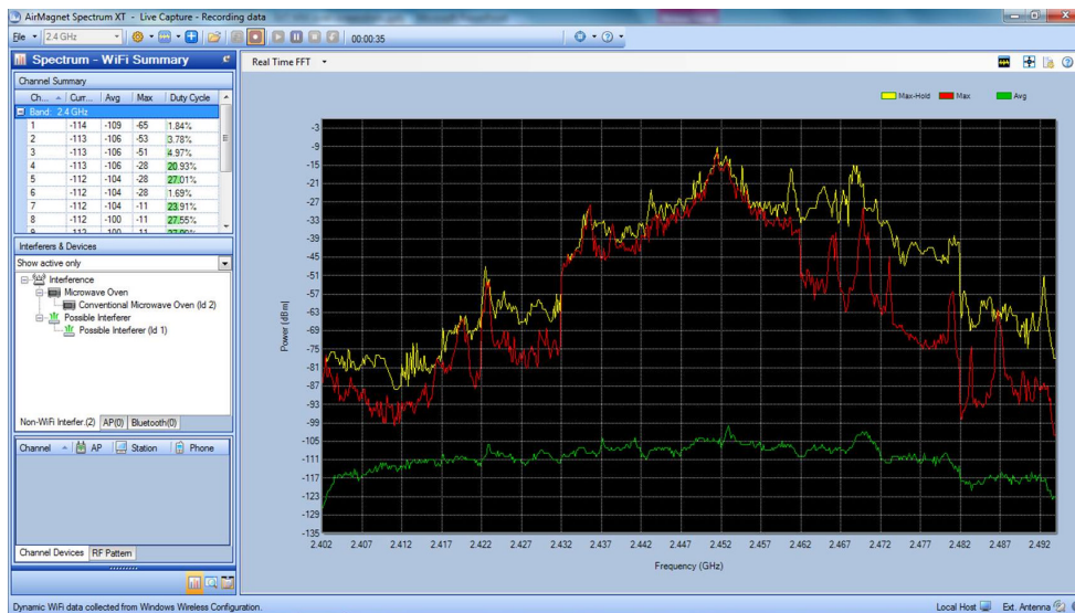
FIGURE 16.2 Microwave oven spectrum use
