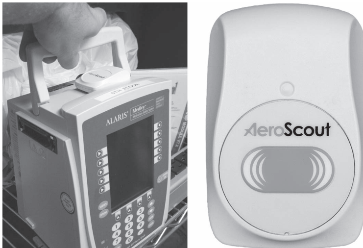
FIGURE 10.28 Active 802.11 RFID tag
