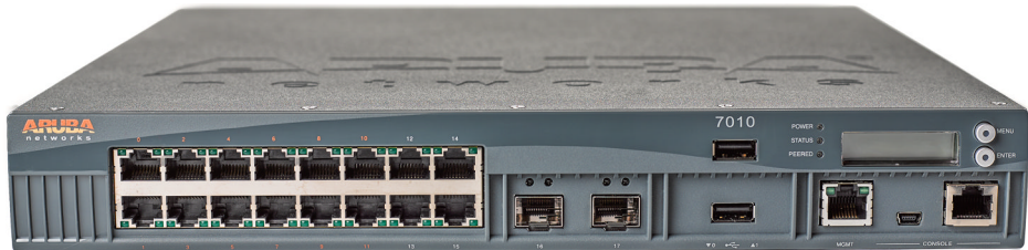
FIGURE 17.2 An Aruba 7010 wireless controller with PoE
