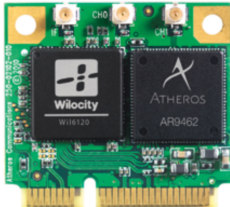
FIGURE 6.3 2.4 GHz, 5 GHz, and 60 GHz tri-band radio card
