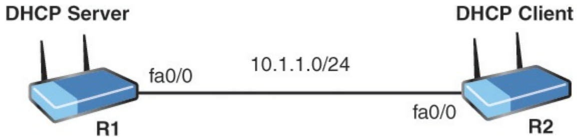
FIGURE 14.2 The DHCP Server and Client Topology
