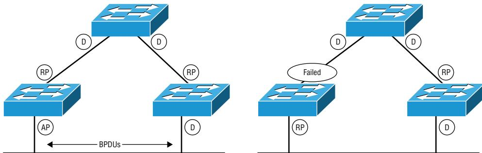
130. C. The root bridge is elected by all of the switches and has the lowest MAC address and priority of all the switches in the network. The root bridge is not elected based upon a high or low IP address. Spanning Tree can function without an IP address, since it is a layer 2 loop avoidance.
