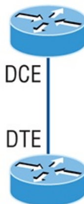
Figure 6-4: Providing clocking on a nonproduction network Set clock rate if needed
