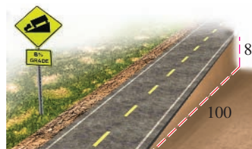
Grade of a road Slope = \frac{8}{100}
