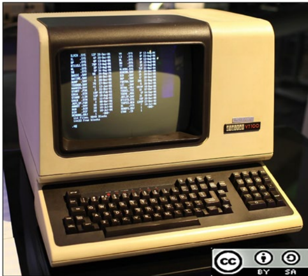
Figure 7-1. A DEC VT100 dumb terminal
