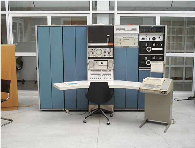
Figure 2-3. A DEC PDP-7 similar to the one used by Ken Thompson and Dennis Ritchie to write the UNICS[sic] operating system. This one is located in Oslo, and the picture was taken in 2005 before restoration began. Wikimedia, CC by SA 1.0
