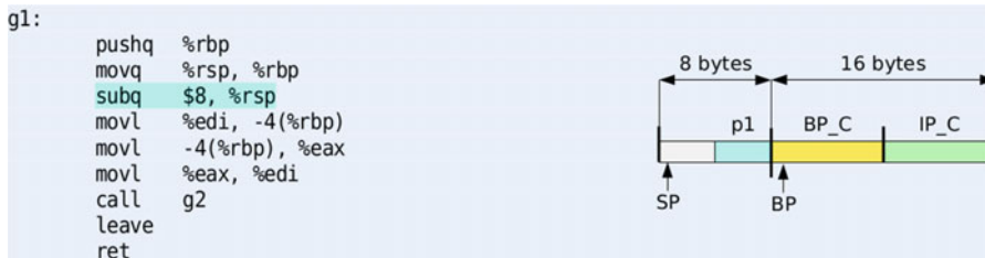
Figure 5-20. Stack frame of g1() ; it doesn't use the red zone. The stack pointer is not properly aligned
