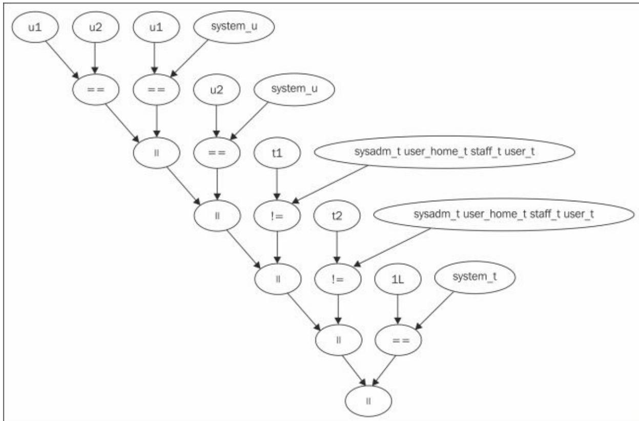
This graph shows how the UBAC constraints are constructed. File reads are prohibited (regardless of the type enforcement rules that are made in the policy), unless they match one of the rules shown in the graph, which are as follows:
