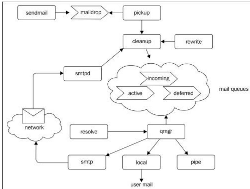
The **smtpd** daemon handles the reception of an e-mail through the **network**, and as such, is more prone to remote vulnerability exploits than to locally running processes such as the **cleanup** process or even the **qmgr** process.
