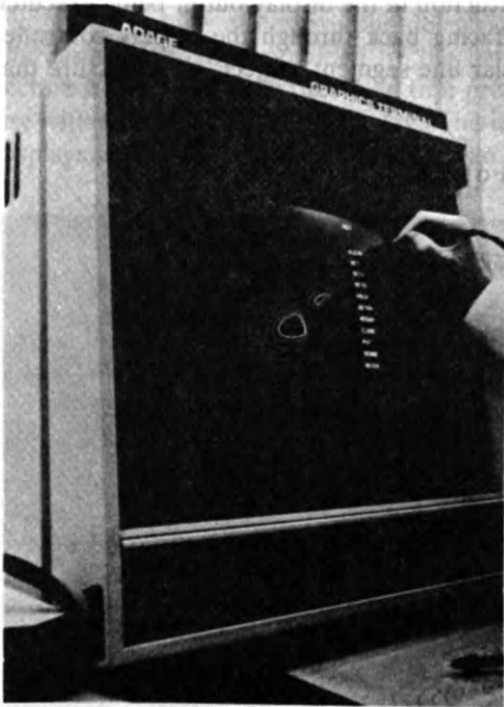
Figure 1-29 A light pen used to simulate a logical button function via menu picking. (Courtesy of Adage, Inc.)
