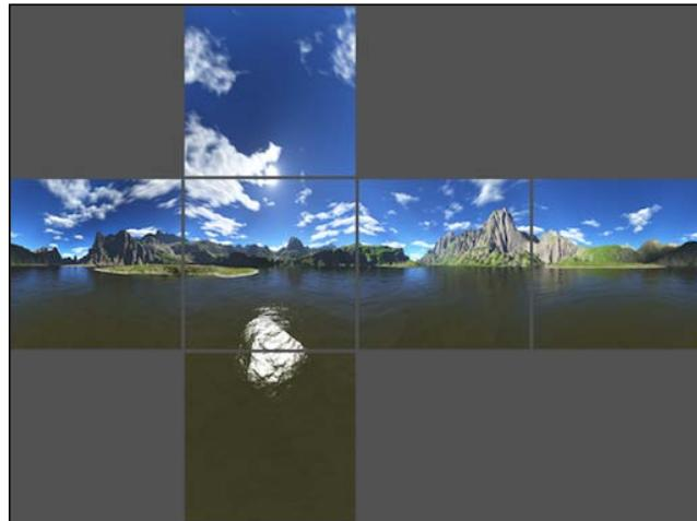
OpenGL provides built-in support for cube map textures (using the `GL_TEXTURE_CUBE_MAP` target). The texture is accessed using a 3-dimensional texture coordinate ( $s, t, r$ ). The texture coordinate is interpreted as a direction vector from the center of the cube. The line defined by the vector and the center of the cube is extended to intersect one of the faces of the cube. The image that corresponds to that face is then accessed at the location of the intersection.
