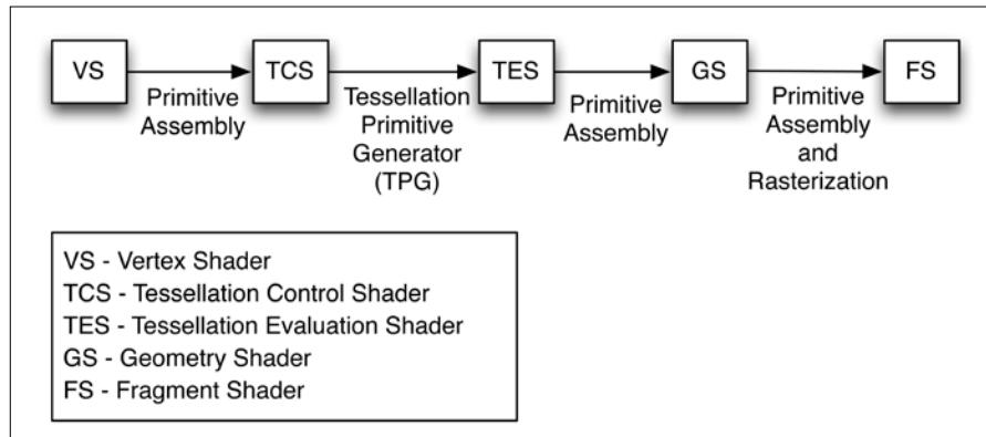
The tessellation portion of the shader pipeline includes two stages: the **tessellation control shader (TCS)**, and the **tessellation evaluation shader (TES)**. The geometry shader follows the tessellation stages and precedes the fragment shader. The tessellation shader and geometry shader are optional; however, when a shader program includes a tessellation or geometry shader, a vertex shader must be included.
