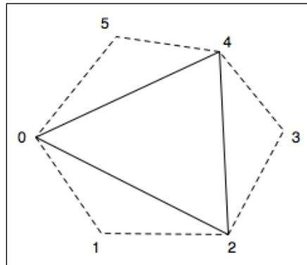
In the preceding diagram, the solid line represents the triangle itself, and the dotted lines represent adjacent triangles. The first, third, and fifth vertices (**0**, **2**, and **4**) make up the triangle itself. The second, fourth, and sixth are vertices that make up the adjacent triangles.
