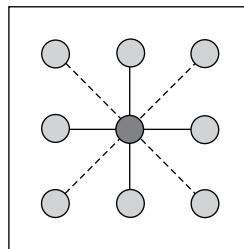
The total force on a particle is the sum of the forces produced by the eight springs to which it is connected. The force for a single spring is given by the following equation:
