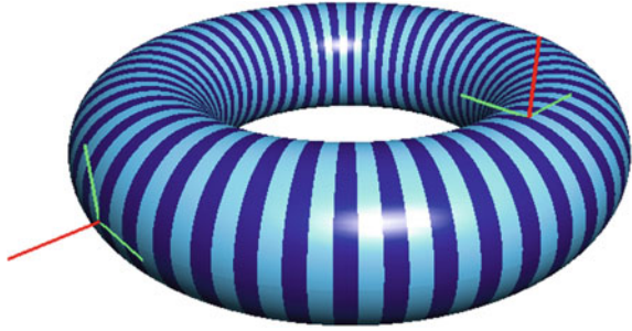
Fig. 13.19 The tangent vectors (green) and normal vector (red) on the left are for \theta = \phi = 0 . The vectors on the right are for \theta = \phi = \pi/2
