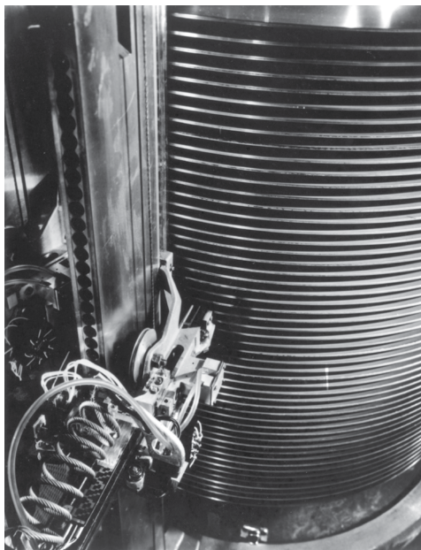
FIGURE 1.8 IBM RAMAC disk storage device, circa 1956
