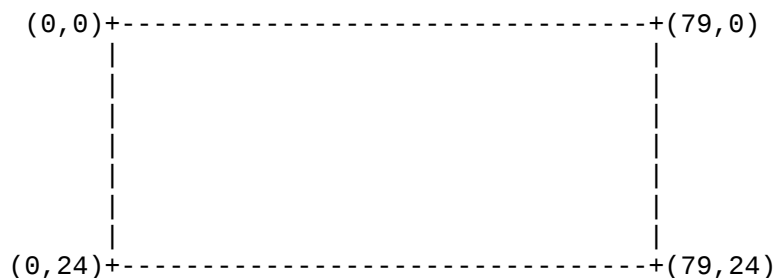
Figure 6-3. Cursor addressing for 80-by-25 text display modes (IBM ROM BIOS modes 2, 3, and 7).
