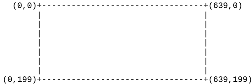
Figure 6-7. Point addressing for 640-by-200, 2-color graphics modes on the CGA, EGA, MCGA, and VGA (IBM ROM BIOS mode 6).
