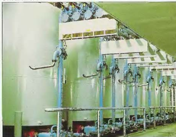
Intermediate holding vats. The conched chocolate is stored temporarily in huge containers kept at a temperature between 113 and 131°F. The chocolate is kept in motion by mechanical or pneumatic means to prevent the cocoa butter from settling.
