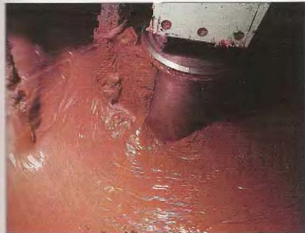
Conching is a refining process that converts the chocolate liquor into a creamy liquid by continuous kneading and through the heat generated by friction. After several hours, the crumbly chocolate liquor turns into liquid chocolate.
