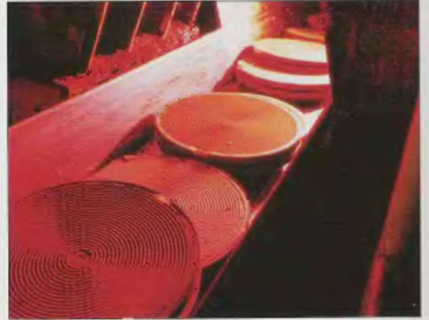
The round cocoa cakes drop from the press directly onto the conveyor belt, which transports them to the crushers. There they are broken into pieces the size of hazelnuts and later ground into powder.
