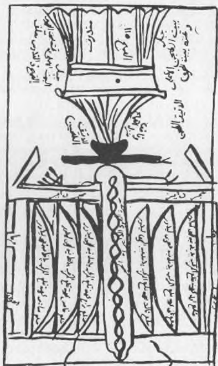
A Seistan windmill of the tenth century. From The Cosmography of Dimashqi , © 1300, reproduced in Rex Wailes's Horizontal Windmills .
