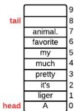
Figure 1. Words stored in a queue. Each word is added to the queue at the tail position and will be removed from the queue at the head position.
