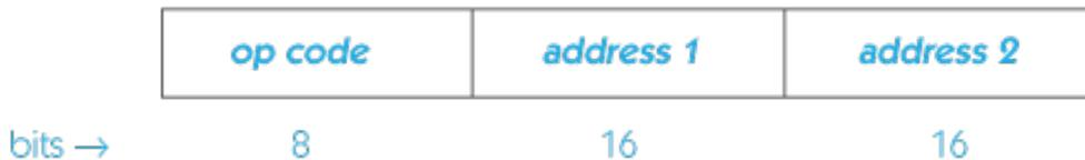
A decimal 9, in 8-bit binary, is 00001001. Address 99, when converted to an unsigned 16-bit binary value, is 0000000001100011. Address 100 is 1 greater: 0000000001100100. Putting these values together produces the instruction ADD X, Y as it would appear in memory:
