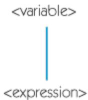
does not generate any machine language code. This branch of the tree is really just the renaming of a nonterminal to avoid the ambiguity problem discussed earlier. This demonstrates an important point: Although most branches of a parse tree produce code, some do not. Although no code is produced, the compiler must still create a semantic record for the new nonterminal <expression>. It is identical to the one built for the nonterminal <variable>.
