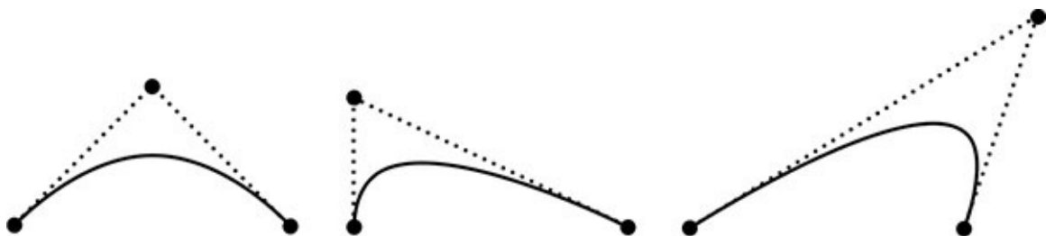
Figure 4-8: Curves defined by two end points and one control point
