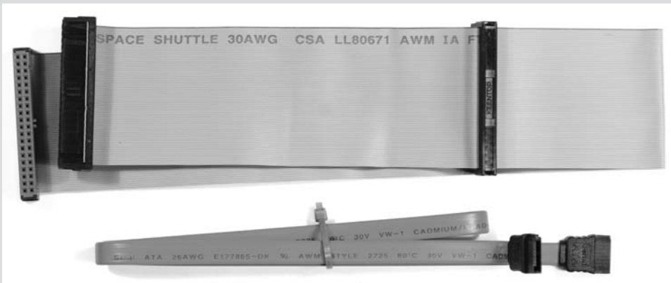
FIGURE 8.25 Parallel ATA (top) and Serial ATA (bottom) cables
