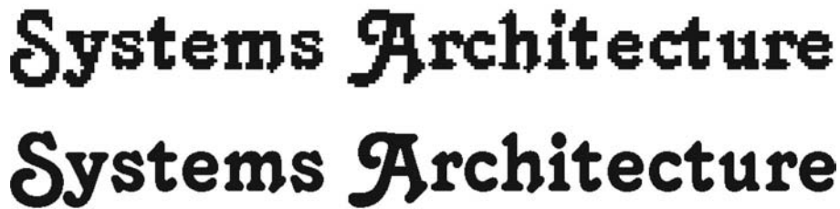
FIGURE 7.2 Text displayed in two resolutions: 50 dpi (top) and 200 dpi (bottom)
