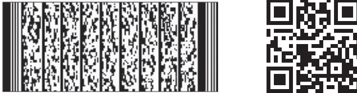
FIGURE 7.15 Two-dimensional bar-code formats
