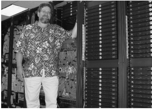
FIGURE 4-27 One of the authors, R. Miller, standing next to several racks of a computational cluster. Notice the racks on the right side of the image consist of a large number of 2U computational units. The three racks on the left and behind R. Miller consist primarily of networking equipment and cables that provide connectivity within the cluster.
