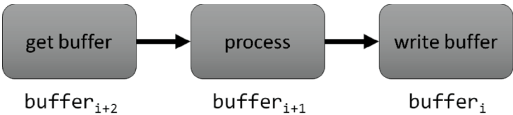
(a) Three buffers processed in parallel by different filters.
