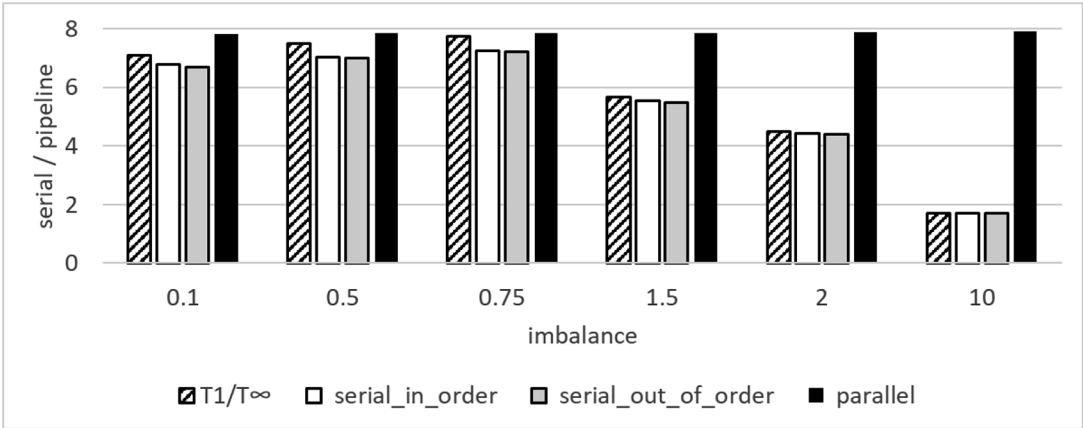
Figure 11-47. The speedup achieved by the different filter execution modes when executing an imbalanced pipeline with eight filters, 8,000 items, and different imbalance factors. Seven of the filters spin for 100 microseconds, and the other spins for \text{imbalance} \times 100 microseconds
