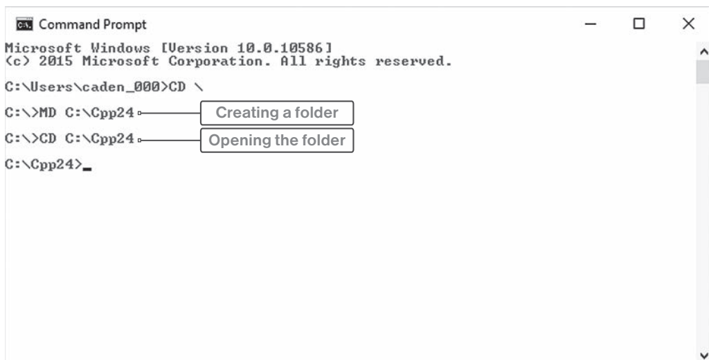
FIGURE D.6 Creating a new folder in a command-line window.
