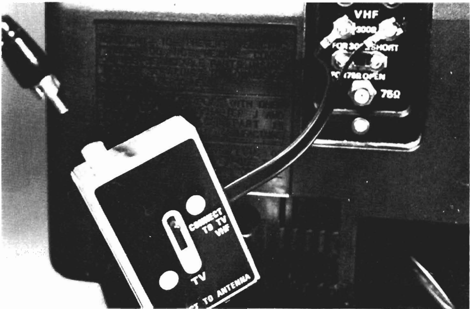
FIGURE 1-4. Television switch box and connections
